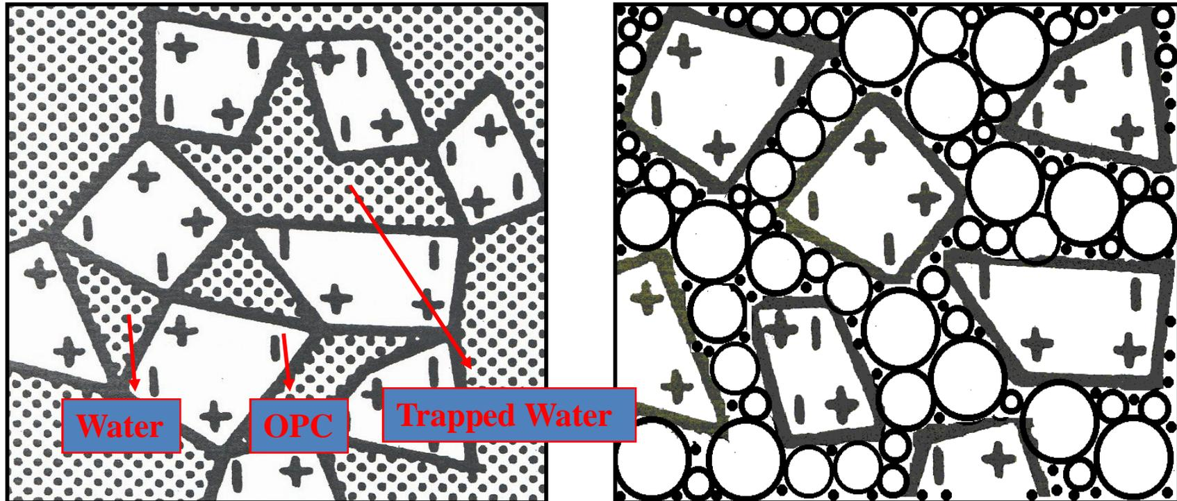
Presence of electronic charges, on Portland cement particle surface, tend to form flocks that trap large volumes of water
