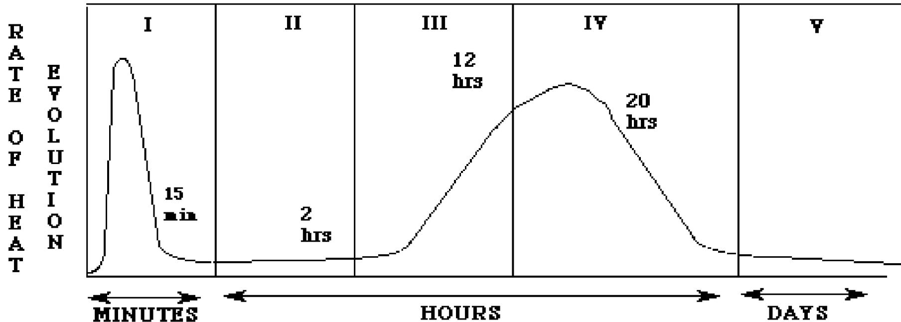
Liberation of Heat is linked to chemical activity, this further affects hardening process. Please note the high exothermic activity at start, gypsum cooling and exothermic activity close to final setting.
