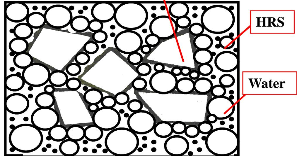
Reduction in inter-affinity between OPC particles due to Ball Bearing Effect provided by HRS
